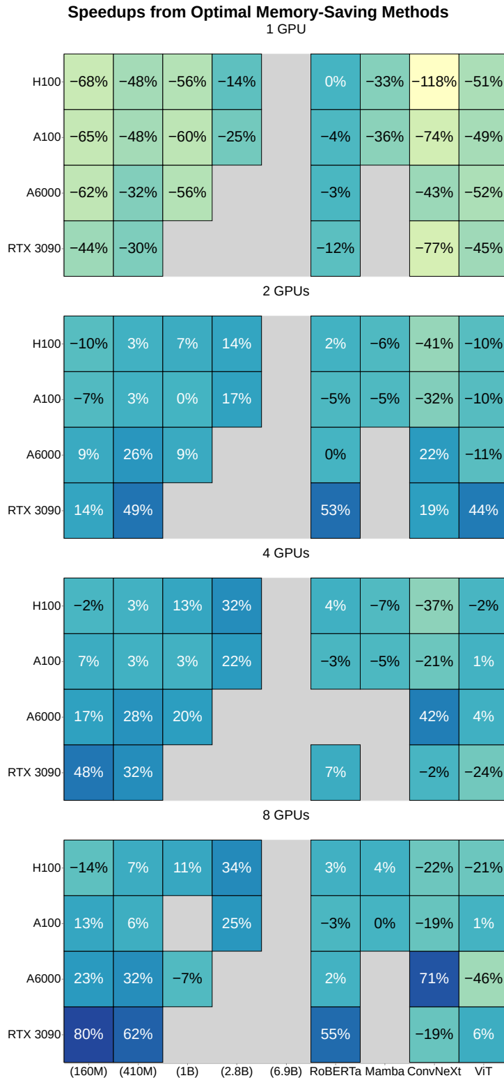
Figure 11: Training time speedups (or slowdowns if negative) for optimal memory-saving methods over using no memory-saving methods (i.e. only free-lunch). Results are shown for our full set of models and deaggregated by number of GPUs. Parenthesized sizes refer to Pythia models. Gray indicates infeasibility when using free-lunch methods alone (and sometimes with all memory-saving methods). As in Fig. 4, we see consistent degradations when using these methods in the 1 GPU setting (where model sharding is a no-op). Here, we can also see that these methods don't benefit the particular computer vision models selected in our investigation as strongly. These models simply require less memory than Pythia (even at similar parameter sizes, due to other differences in hyper-parameters e.g. in sequence length and batch size). Thus, they see fewer benefits from memory-saving methods.
